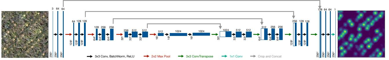
Figure 2: Our architecture follows the encoder-decoder structure of U-Net where the input is an RGB image and the output is a density map.
